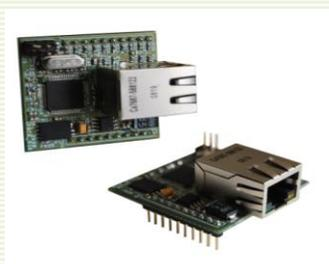
The Gateway module IPACK P-401, dedicated component for IP access, developed by the Spanish company IPLógiKa is hardware platform for the Ethernet access based on an embedded microprocessor.
