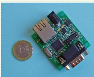
The RS232 Gateway Module IPACK P-402, dedicated component for IP access, developed by the Spanish company IPLógiKa is hardware platform for the Ethernet access based on an embedded microprocessor.
